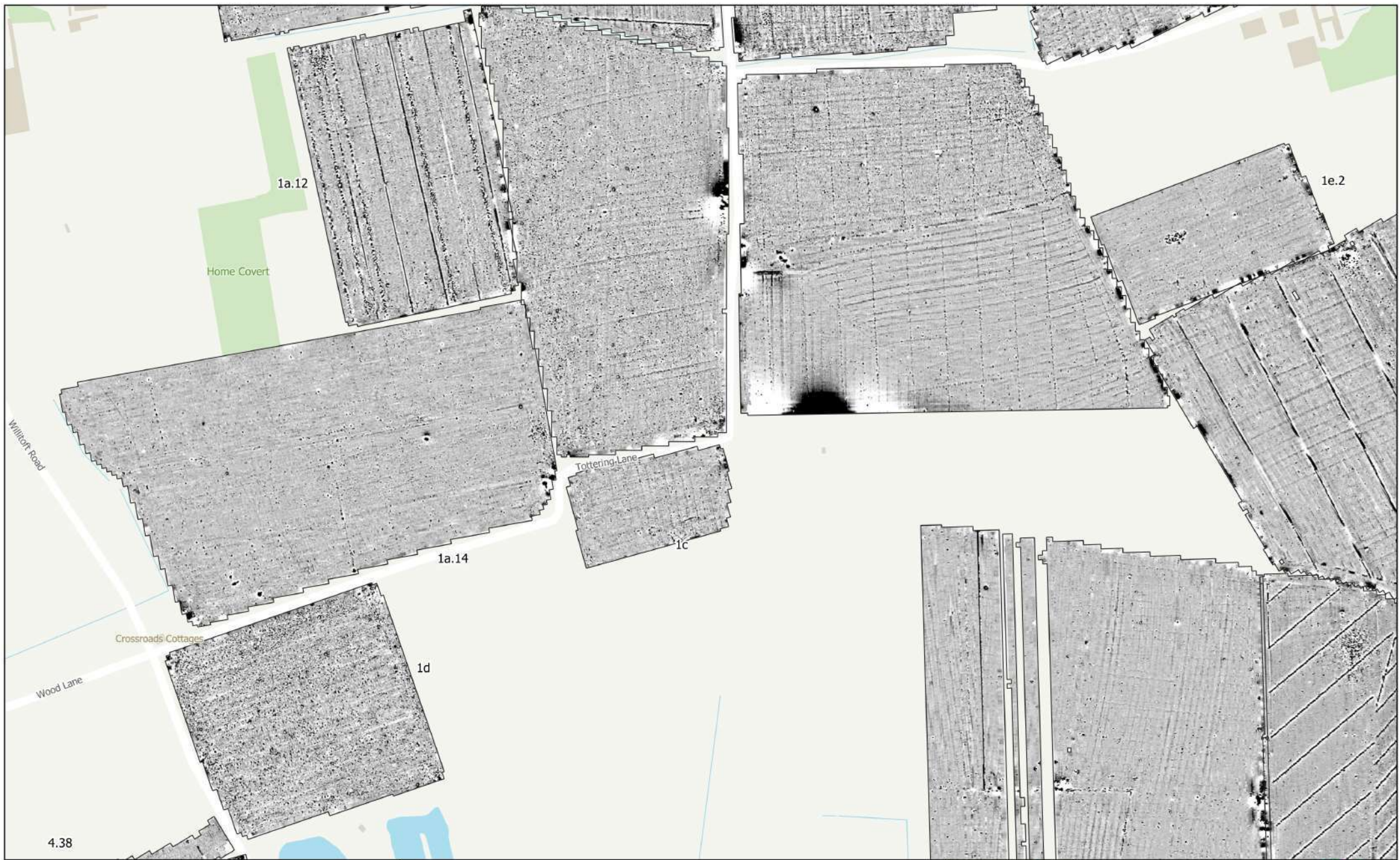
MSSE1401 - East Yorkshire Solar Farm Figure 10 - Magnetic Gradient (Areas 1a.12, 1a.14, 1c, 1d, 1e.2 and 1e.3) 1:4,000 @ A3 Copyright Magnitude Surveys Ltd 2023 Contains Ordnance Survey data © Crown Copyright and database right 2023
