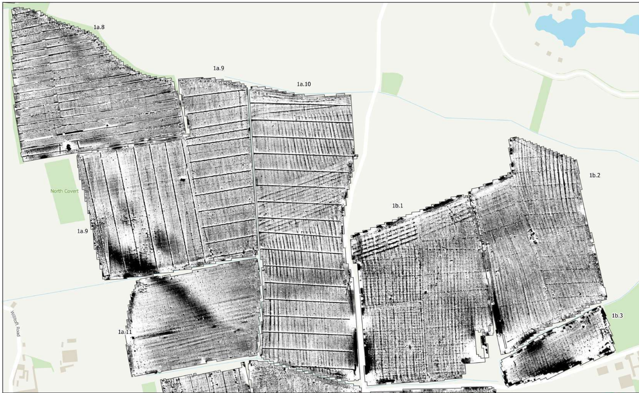
MSSE1401 - East Yorkshire Solar Farm Figure 6 - Magnetic Total Field (Lower Sensor) (Overview) (Areas 1a.8 to 1b.3) 1:4,000 @ A3 Copyright Magnitude Surveys Ltd 2023 Contains Ordnance Survey data © Crown Copyright and database right 2023
