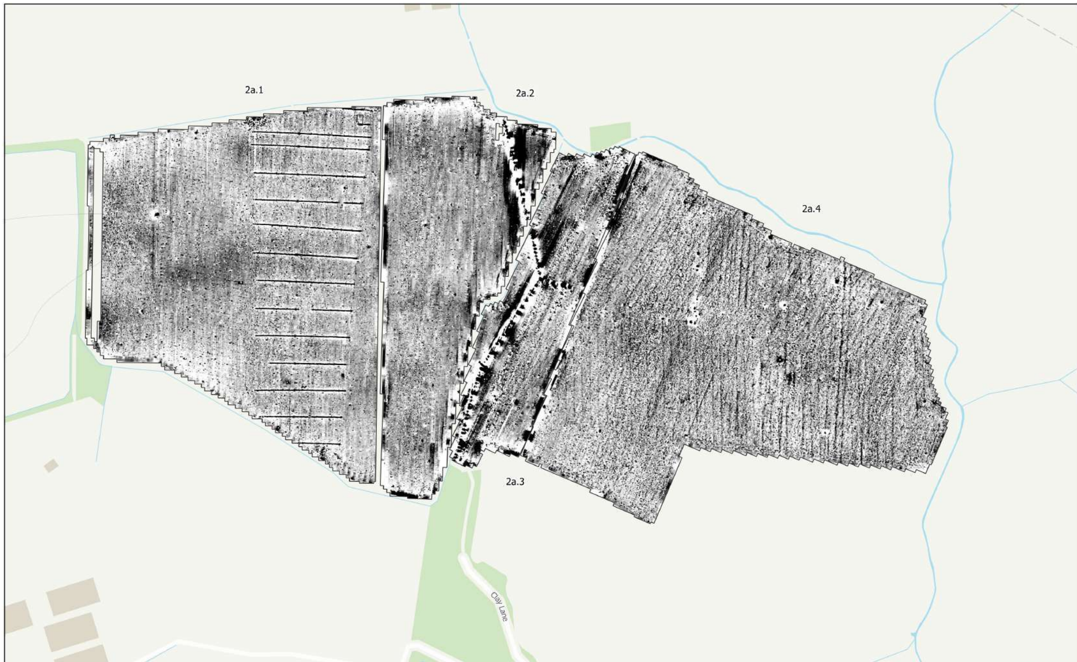
MSSE1401 - East Yorkshire Solar Farm Figure 30 - Magnetic Total Field (Lower Sensor) (Overview) (Areas 2a.1 to 2a.4) 1:4,000 @ A3 Copyright Magnitude Surveys Ltd 2023 Contains Ordnance Survey data © Crown Copyright and database right 2023
