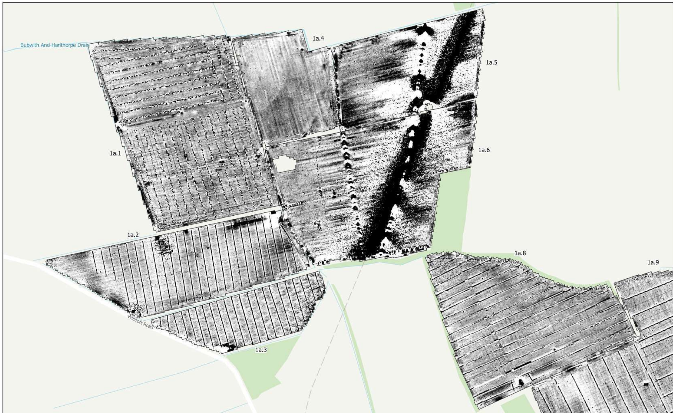
MSSE1401 - East Yorkshire Solar Farm Figure 3 - Magnetic Total Field (Lower Sensor) (Overview) (Areas 1a.1 to 1a.9) 1:4,000 @ A3 Copyright Magnitude Surveys Ltd 2023 Contains Ordnance Survey data © Crown Copyright and database right 2023
