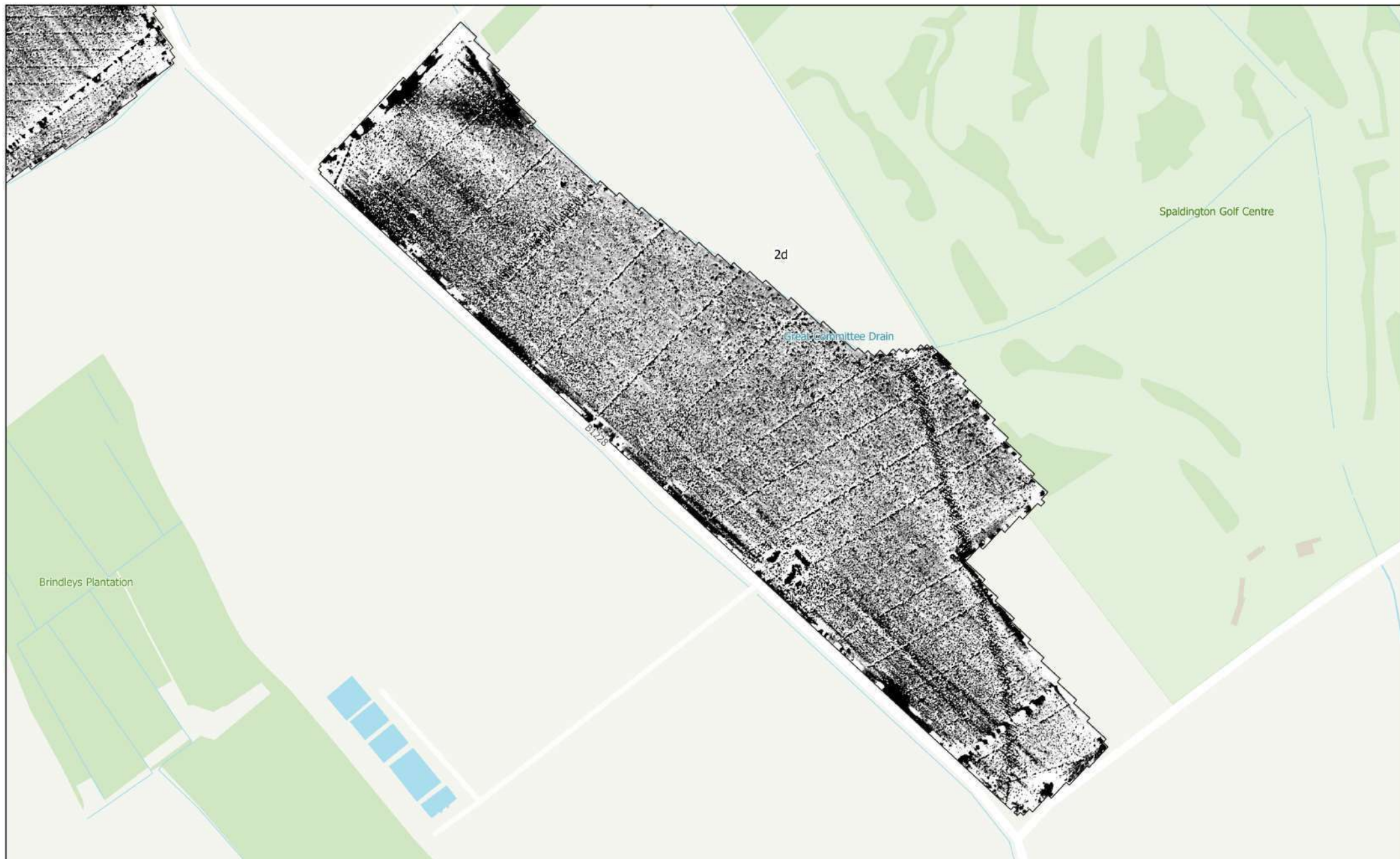
MSSE1401 - East Yorkshire Solar Farm Figure 39 - Magnetic Total Field (Lower Sensor) (Overview) (Areas 2c and 2d) 1:4,000 @ A3 Copyright Magnitude Surveys Ltd 2023 Contains Ordnance Survey data © Crown Copyright and database right 2023
